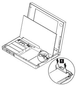
**Note:** After replacing the hard disk drive, latch the removal strap into the correct position.
